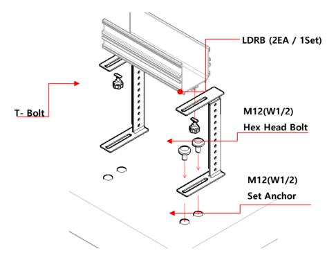
LDRB is designed as adjustable assembly parts with considering the limited height at working place. Assembling Sequence for LDRB is as below.
