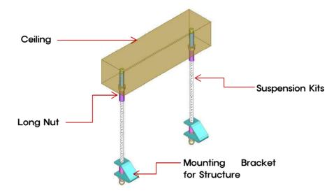
1. After assembling Suspension kits, please put Structure, and then firmly fasten the nut of Mounting Bracket. Further, the Connection among Structure uses Structure Joiner as below.
